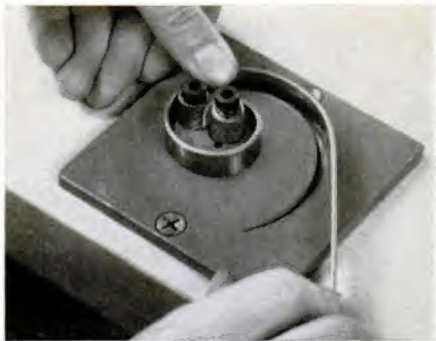
TO BEND CURLS , studs on scroller grip metal strip so you can wrap it around raised spiral on plate
